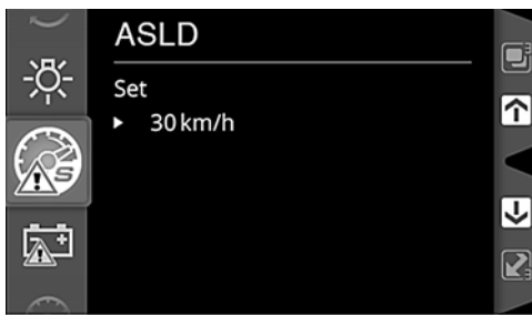
1. ASLD (over speed warning) setting
