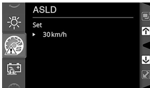
1. ASLD (over speed warning) setting
