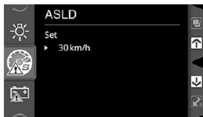
1. ASLD (over speed warning) setting
