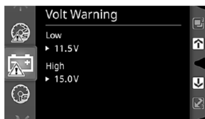
1. Voltage warning setting
