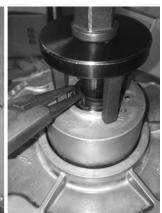
Disassemble the cam, spring, spring seat and outer haft sheave.
