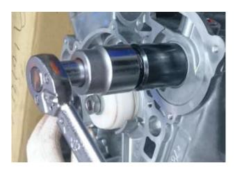
**NOTICE:** After installed, Clean and remove the overflow of glue to prevent block the shaft motion.
