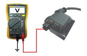
• Check for resistance between the ignition coil connector terminal and ground.
