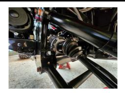
Remove securing the differential bolts and nuts.
