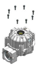
Apply rubber hammer lightly knock the case to separate the half case.
