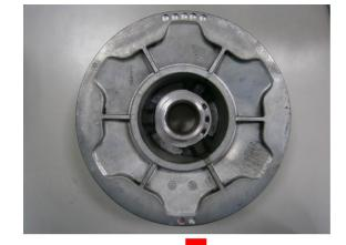
**NOTE:** The hole of spring seat should align the hole of outer haft sheave.
