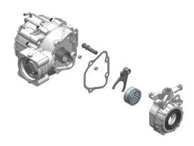
• Install the lock sleeve and shift rod.
