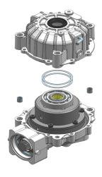
• Check the bearing, replace if necessary.
