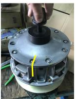
• Loosen ten bolts on the tuner cover.
