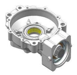
Apply Loctite #263 on the eight bolts and cross tighten.
