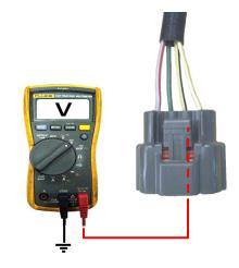
Measure the voltage between the connector terminals of wire harness side.
