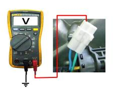
Crank the engine with the starter motor, and measure the crank position sensor peak voltage at the crank position sensor 2P connector.
