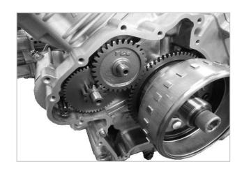
**NOTE:** Use grease to place protector on crankshaft end prior to screw on the FLYWHEEL REMOVER.
