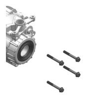
Apply Loctite #263 on the bolts and cross tighten as shown.
