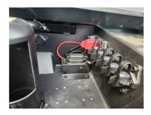
To remove fuse box cover, simultaneously squeeze tabs inwards on each end of fuse box cover as you pull upward on the cover.
