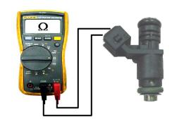
Check for continuity between the injector and ground.
