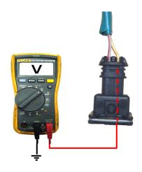
Measure the voltage at ECT sensor connector of the wire harness side.
