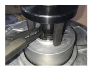
Adjust the open area of two C-clips to perpendicular direction as shown.
