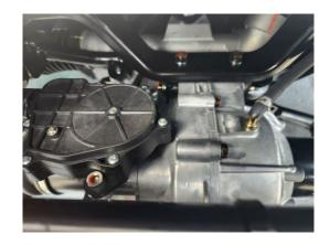
Tighten the upper and bottom front end bolt .
